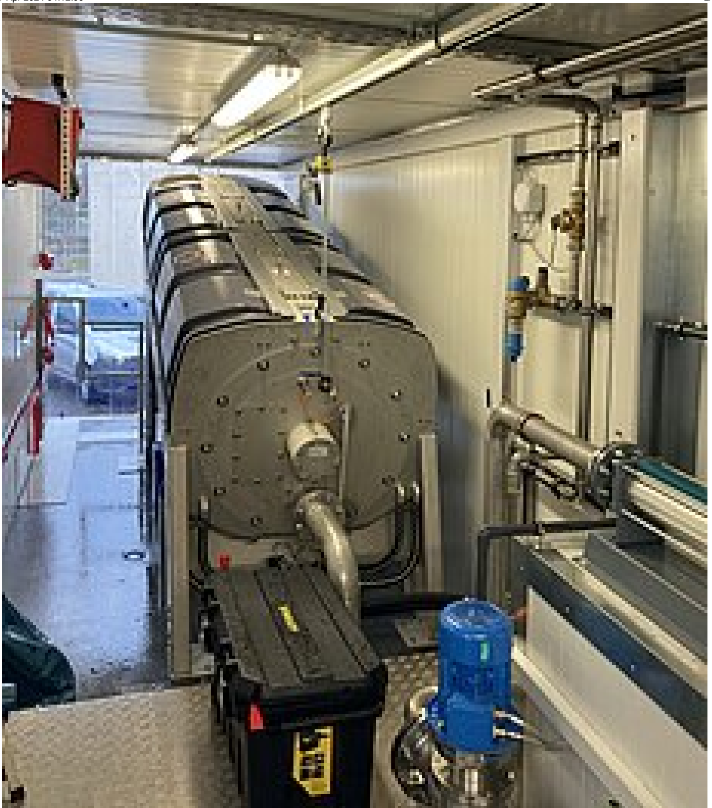
HUBER Screw Press Q-PRESS®, installed in a semi-trailer
