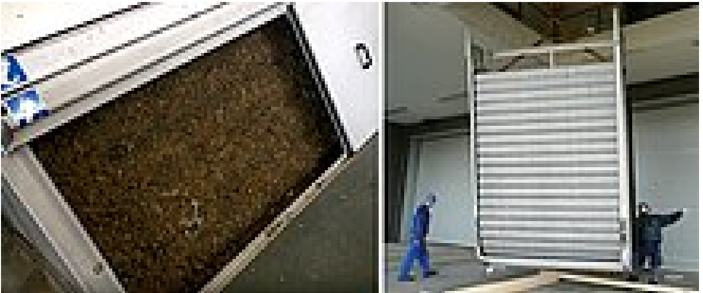
HUBER Belt Screen EscaMax®: Blinding of the screen during load operation and insertion of the bottom part of a two-part HUBER EscaMax® screen into the screen building
