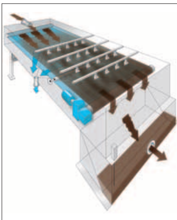
HUBER Drainbelt Uncomplicated, efficient biological sludge thickening
