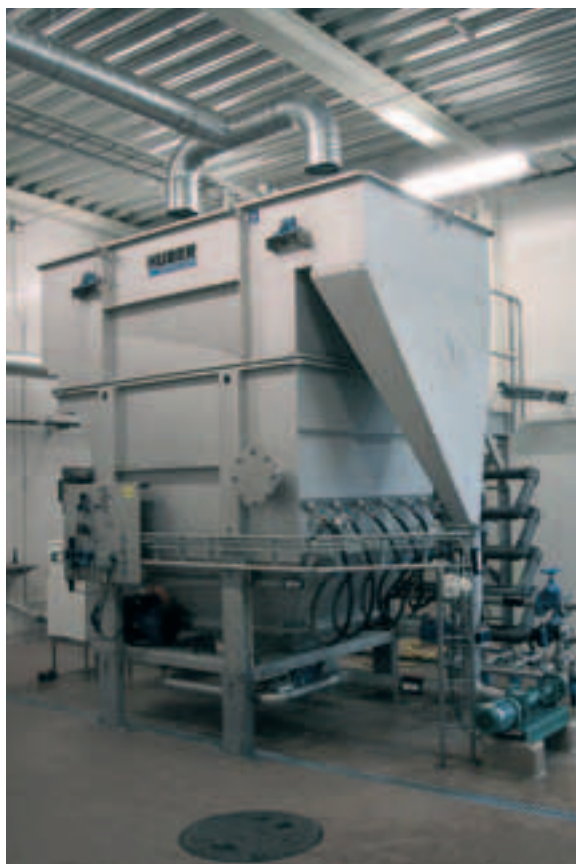
HUBER Flotation Plant HDF with chemical treatment stage for up to 30 m 3 /h
