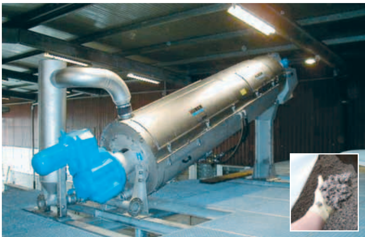
Flotate sludge dewatering with HUBER ROTAMAT® RoS 3 Image detail: Dewatered flotate sludge with > 30 % DS content
