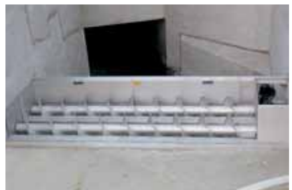
Combination of two HUBER ROTAMAT® RoK 1 Screens to handle very high combined water flows
